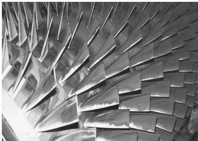
Figure 35. Axial Compressor Online Washed Every Four Days During 744 hours Operation. (Courtesy Turbotec Ltd.)
