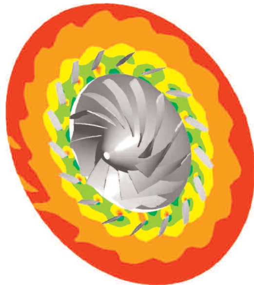
Figure 7. CFD Results Showing Pressure Field Around LSD Vanes.
