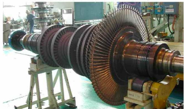
Figure 25. Typical ISB Applied to Mechanical Drive Turbine (After Operation).
