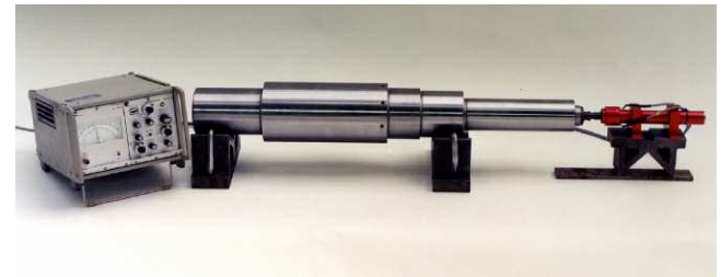
Figure A-2. Test Rotor with Measuring Equipment.
