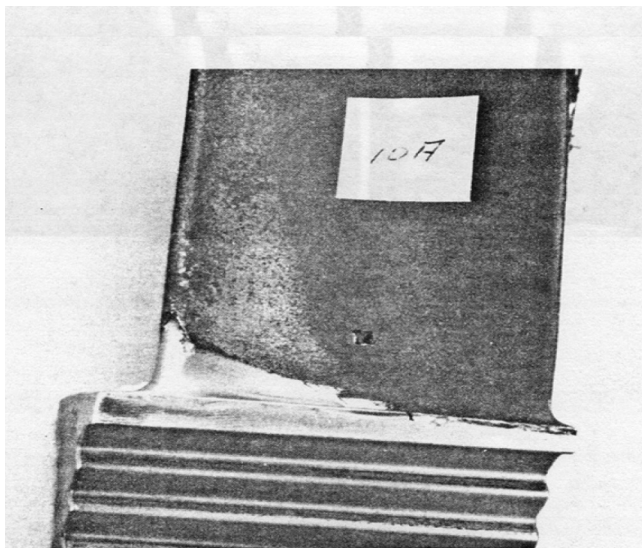
Figure 34. Secondary Erosion of Waspaloy Rotating Blades (B).
