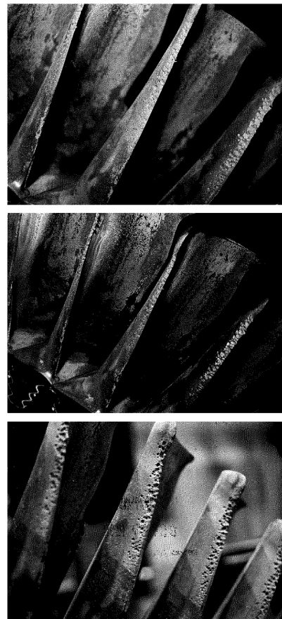
Figure 31. Primary Erosion of Rotating Blades (A).
