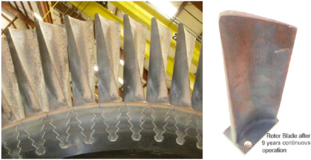
Figure 36. Rotating Waspaloy Blades after Nine Years Continuous Service.
