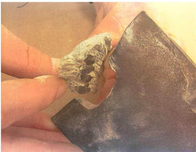
Figure 38. Rub Tip Cracking on Rotating Waspaloy Blade Leading to Material Removal.
