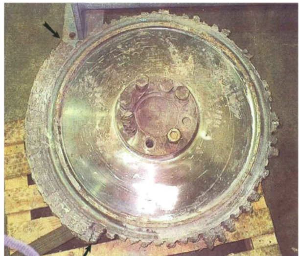
Figure 40. Photograph of Failed First Stage Disk. Arrows Indicate Area Where Disk Tenons Remained Attached.
