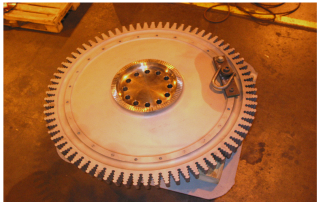
Figure 53. Picture of the Exhaust Face of the Disk.
