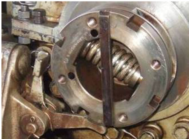
Figure 1. Mechanical Overspeed Trip Mechanism Photo. (Courtesy Younie, 2009)
