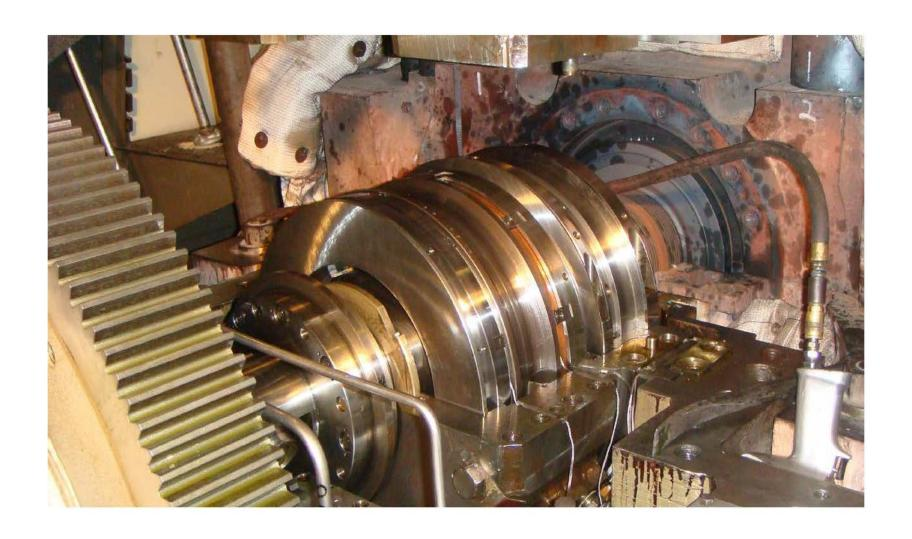
The active thrust bearing after 6 years in service.
