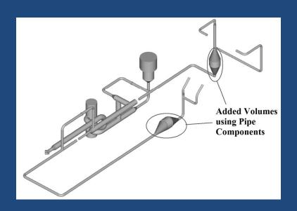
The size of the volumes was selected based on the concept that adding compliance would shift the natural frequency as well as provide some low pass filter effect.
