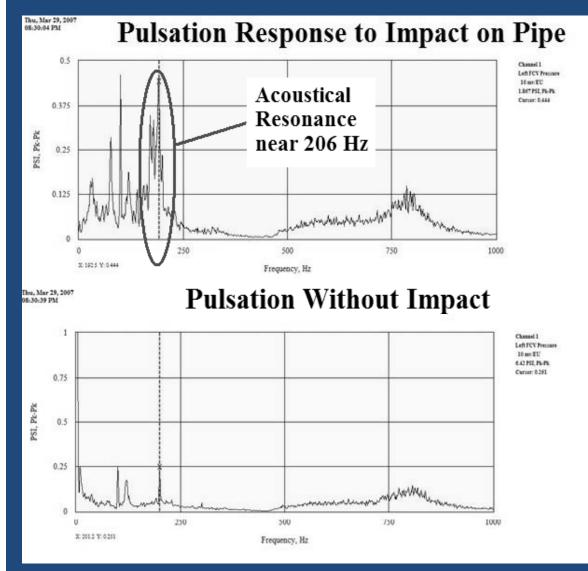
Pressure pulsation sensor installed near one flow control valve suggested that an acoustical resonance existed near 1X pocket pass frequency when pipe impacted with soft mallet.
