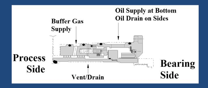
• The seals use were an oil buffered mechanical type. Seal oil was supplied to each seal assembly at approximately 30 PSI above reference gas pressure, using back pressure control valves.
