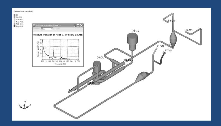
The predicted results were shown to almost eliminate pulsations upstream of the volumes as well as tremendously reducing the reaction at the seal connections at the compressor.
