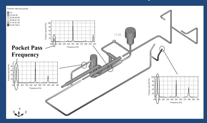
Acoustical analysis of the seal oil supply and return piping was done
