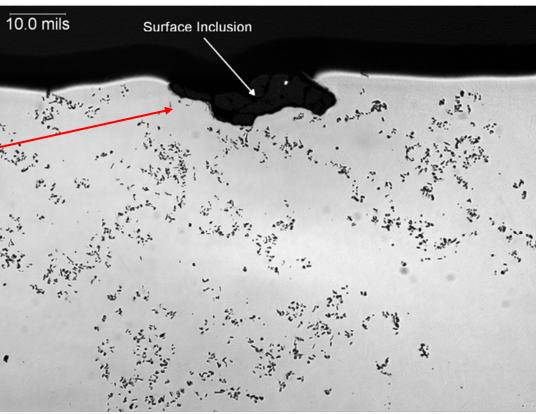
Sub-surface inclusions probably caused by a defect on the casting process
