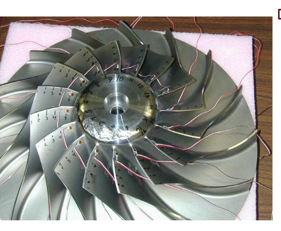
□ As in the case of the first forged impeller, we used strain gages to measure the vibration frequencies
