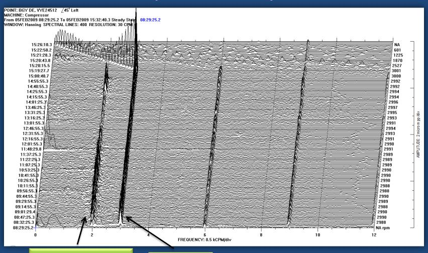
Sub-synchronous vibrations (.147X Pinion)
