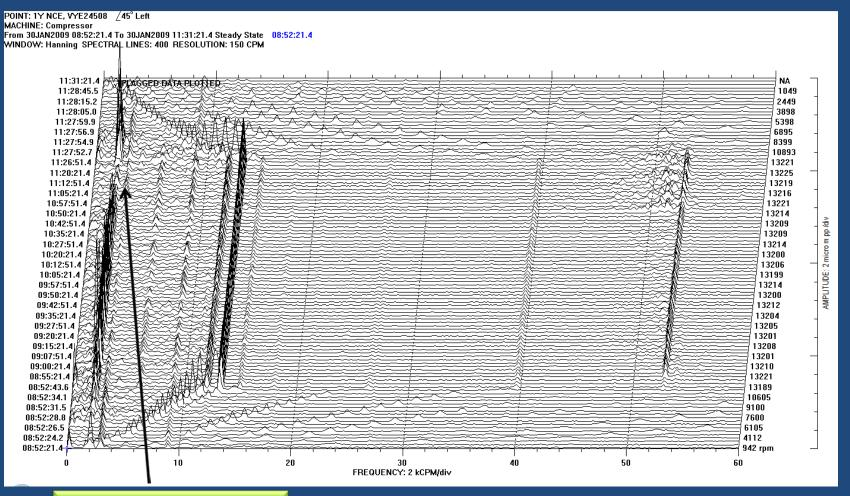
Sub-synchronous vibrations disappeared at closed DGV
