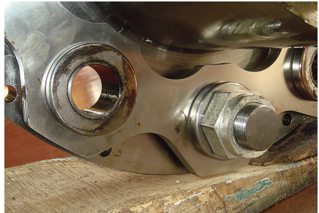
Figure 8. Case 2 Fretting of Disc Pack Washers.
