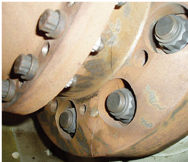
Figure 25. Case 7 Cracked High Performance Disc Coupling.
