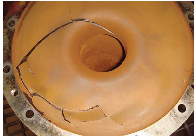
Figure 16. Case 5 Diaphragm Failure Opposite Side.
