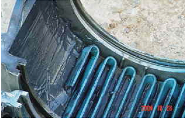
Figure 5. Case 1 Failed Grid Coupling.
