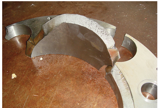
Figure 9. Case 2 Beach Marks at Fracture Site.
