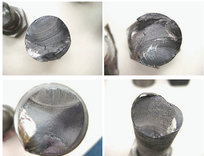
Figure 13. Case 3 Beach Marks on Failed Bolts.
