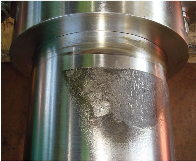
Figure 10. Case 2 Shaft Damage.
