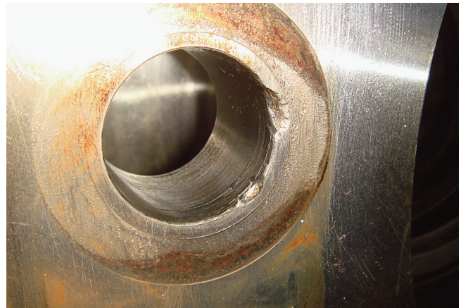
Figure 7. Case 2 Fretting on Disc Pack Flange.
