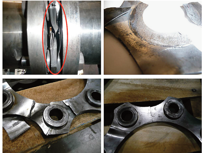
Figure 12. Case 3 Disc Pack Damage.
