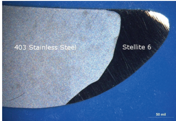
Figure 57. Cross-Section of a 403 Stainless Steel Turbine Blade with Stellite® 6 Weld Overlay.
