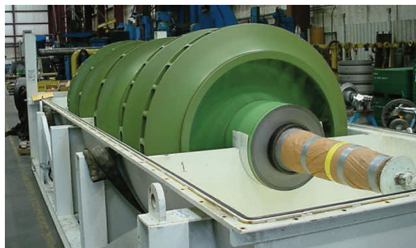
Figure 7. Centrifugal Compressor Rotor Coated with an Organic Antifoulant Coating (Dowson, 2007).
