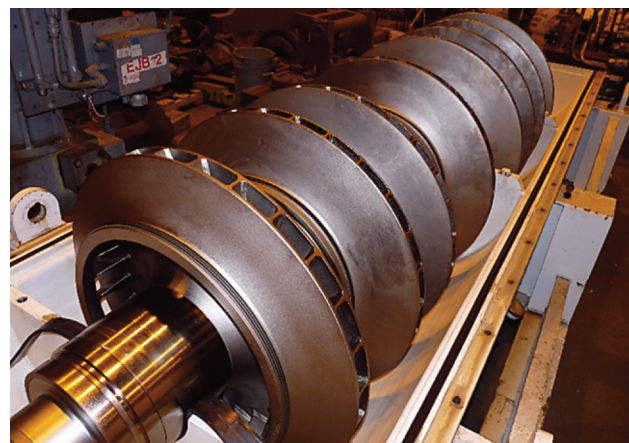
Figure 15. Photo Showing an Electroless Nickel Coated Rotor after Five Years Service.
