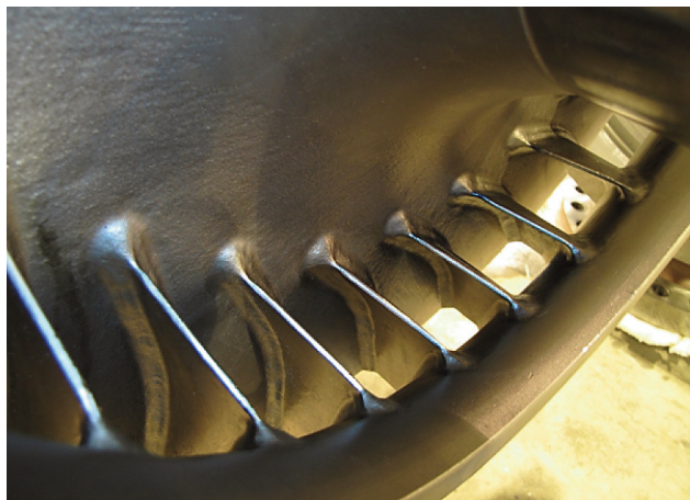
Figure 13. Image Showing Gas Path of a Centrifugal Compressor Impeller Coated with Electroless Nickel.
