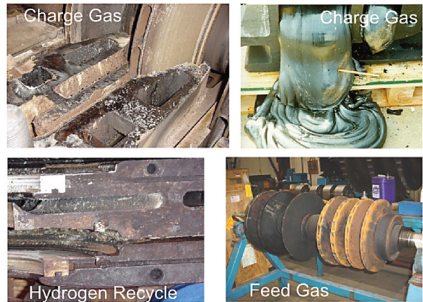
Figure 6. Examples of Fouling of Centrifugal Compressors in Various Services.
