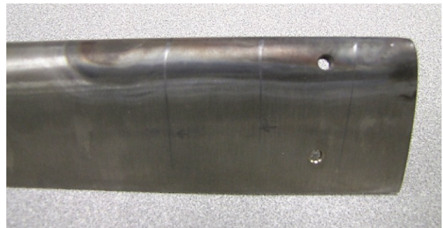
Figure 60. Leading Edge of a Flame Hardened Turbine Blade.
