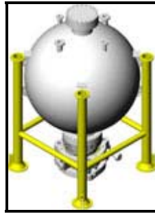
Figure 2.5: A subsea gravity separator 7 .
