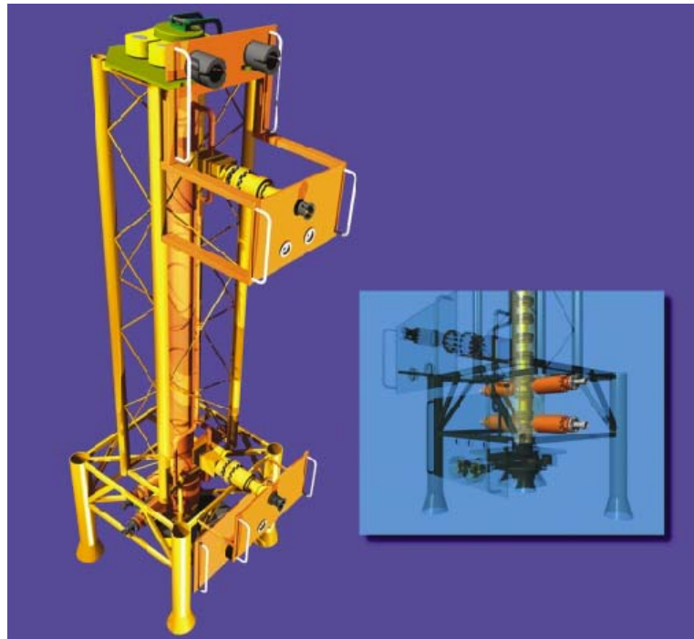
Figure 4.6: Equipment for single trip pigging 24 .
