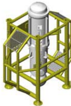
Figure 2.11: Schematic of a subsea gas compressor 5 .
