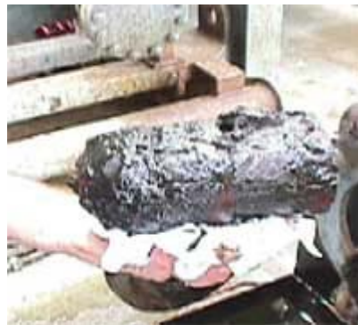
Figure 4.2: An asphaltene plug removed from a pipeline 5 .
