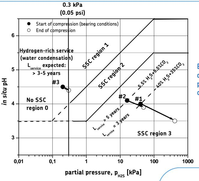
Based on NACE/ISO SSC diagram with working points for compressor cases # 1 to 3
