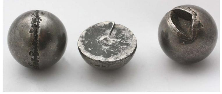
Left: Ball with initiation grove around the equatorial running line. **Middle:** A ball after being split in half under running.
