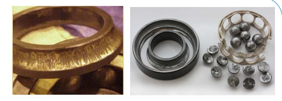
**Ring spalling** of conventional ball bearing rings **by stress cracking from wet sour gas** in combination with standstill periods **Typical sour gas failure** by stress cracking, causing **splitting of conventional steel balls**. Secondary failure of brittle polymeric PPS cage.
