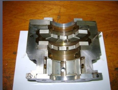
HP Thrust and Radial Bearing No Visible Damage
