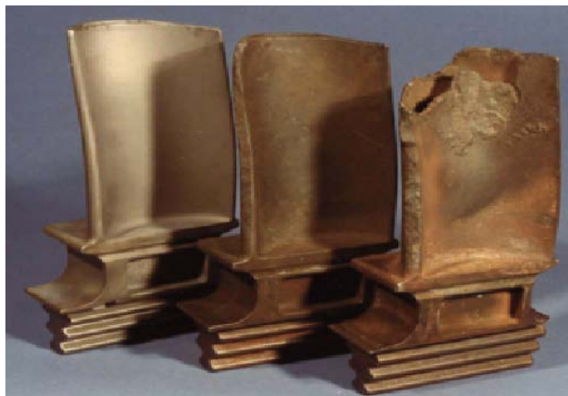
Figure 16: Hot Corrosion on Turbine Blades after about 1,000 hrs of Operation on Distillate Fuel Containing 2 ppm Sodium from Sea Water Contamination (Courtesy Turbotect Ltd. )
