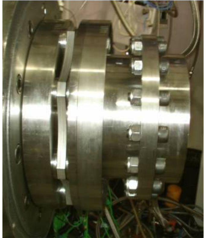
Figure 21. Test rig with drive bolt windage feature.
