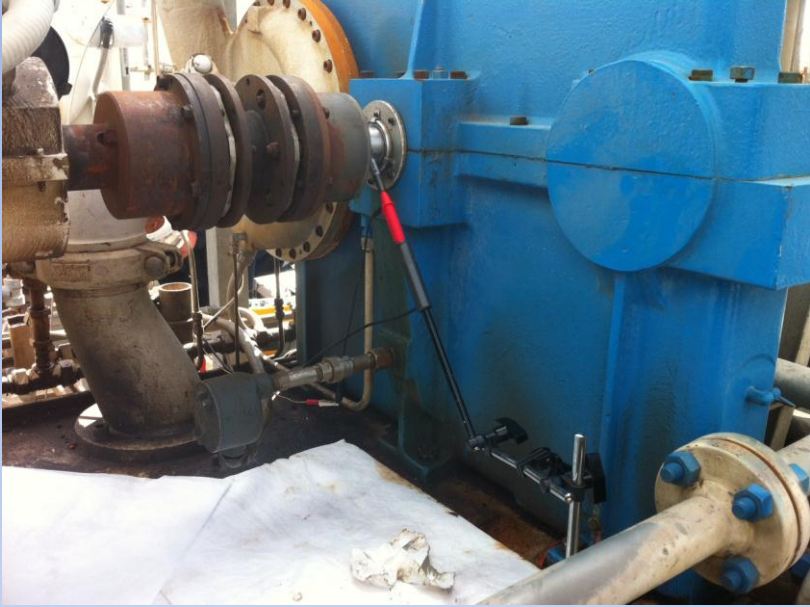
Carbon fiber shaft probe and portable oscilloscope
