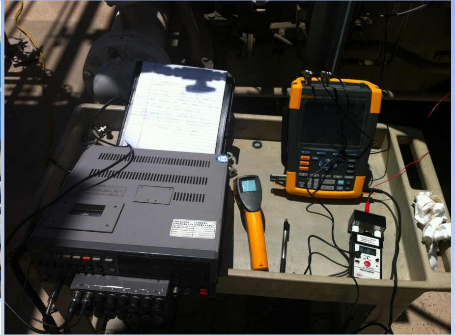
Electro-static charge detector with a charge plate adapter for use with a pipe probe
