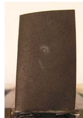
Figure 29. Blade Sprayed with Dirt/Gain/Deionized Water Mixture in Heated Air Stream
