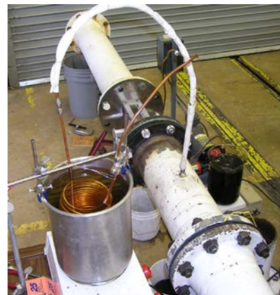
Figure 31. Heated Dirt/Water Injection Setup
