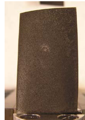
Figure 27. Blade Sprayed with Dirt/High-Purity Deionized Water Mixture in Heated Air Stream
