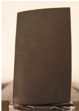
Figure 26. Blade Sprayed with Dirt/Tap Water Mixture in Heated Air Stream
