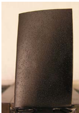
Figure 28. Blade Sprayed with Dirt/Commercial Detergent Mixture in Heated Air Stream
