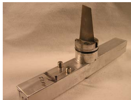
Figure 11. Blade Mounting Fixture with Blade Installed
