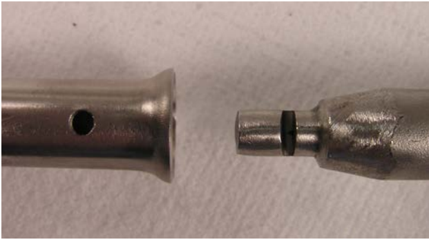
Figure 16. Flow Blockage Tube (Left) and Nozzle (Right)
