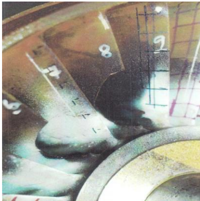
Figure 28 Photograph showing Thumb Nail or Scallop Fatigue Cracks in an Impeller
