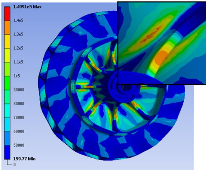
**Figure 7. 2<sup>nd</sup> Generation 0.11  $\phi$ , Ti-6Al-4V Impeller – Von Mises Stress (psi) at 37,830 rpm**
