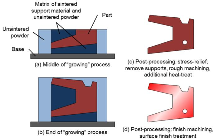
**Figure 1. Illustration of DMLS Process**
