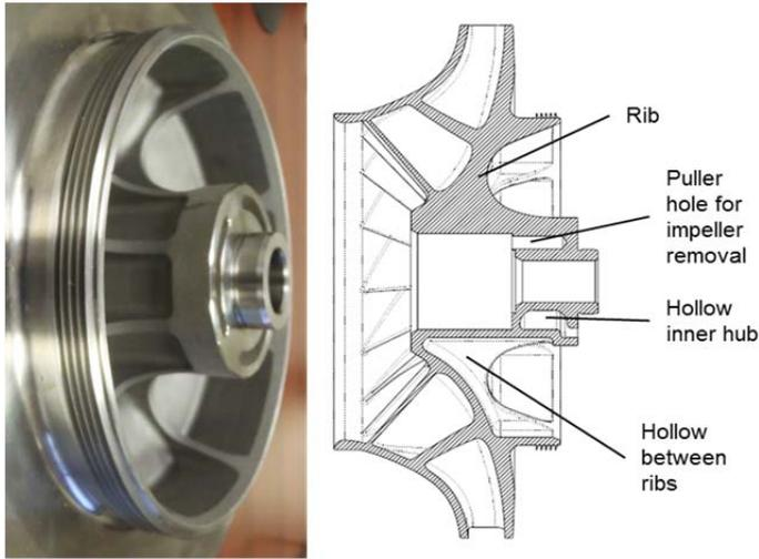
**Figure 4. Thinner Cross-Section Hub Design Required for Titanium Impeller**
