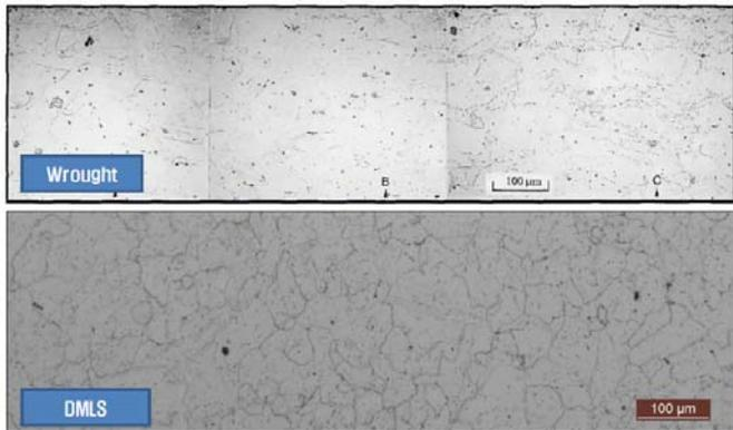
Figure 13. Comparison of Grain Size Between Wrought Inconel 718 and DMLS Inconel 718
