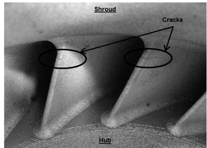
**Figure 3. Cracks at Blade Leading Edge Due to Heat Treatment of 1<sup>st</sup> Generation 17-4 PH Stainless Steel Impeller**
