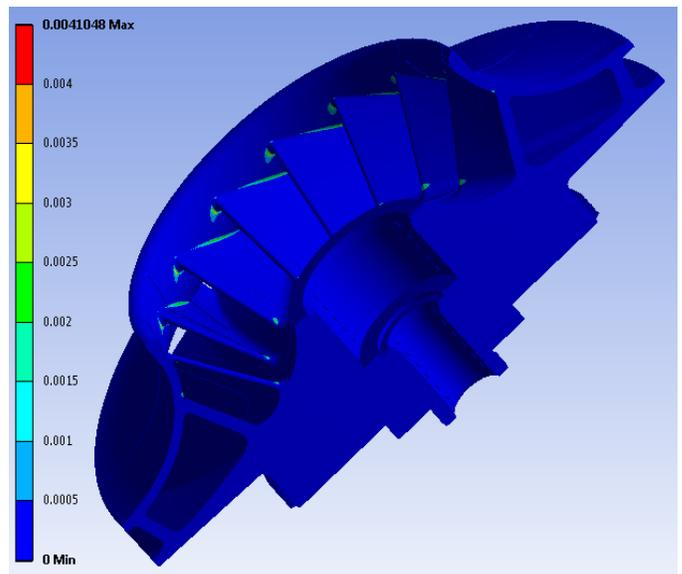
**Figure 6. Elastic-Plastic Analysis Plastic Strain Results for 2<sup>nd</sup> Generation 0.08  $\phi$  Impeller, Overspeed Condition**
