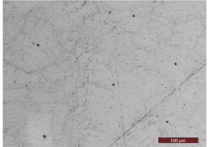
Figure 14. Magnification of DMLS Inconel 718 Sample Showing Micro-Porosity
