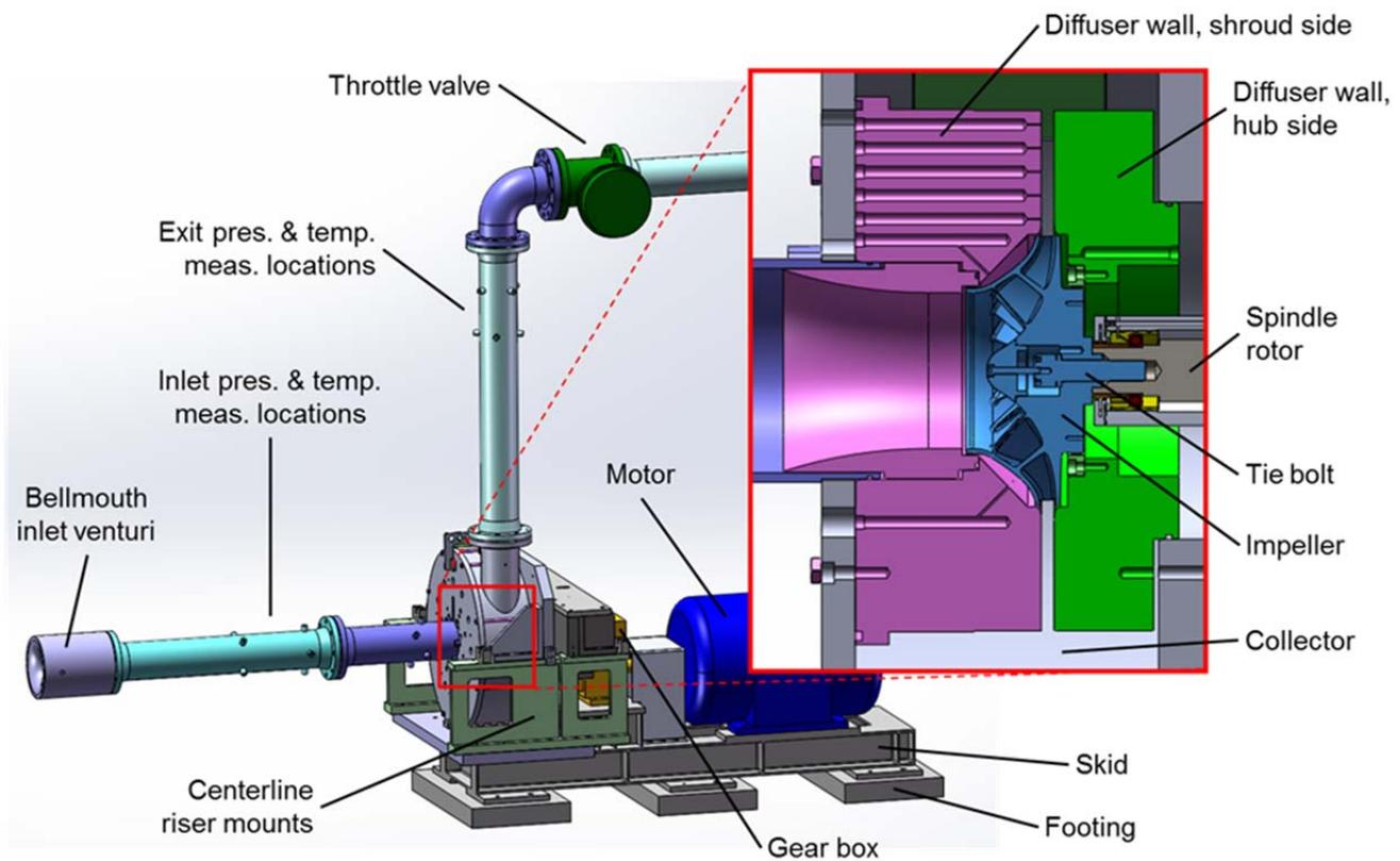
Figure 15. SSTR Layout – Simple Collector Configuration
