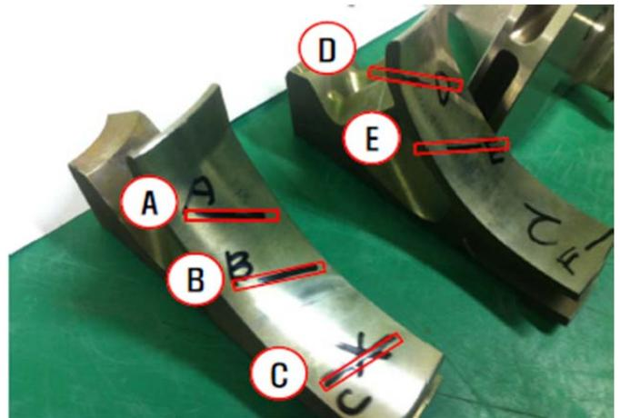
**Figure 10. Sections of 2<sup>nd</sup> Generation DMLS Shrouded Impeller Being Cut for Inspection**
