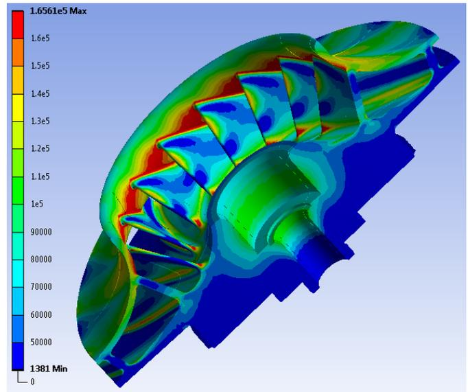
**Figure 5. Elastic-Plastic Analysis Stress Results (psi) for 2<sup>nd</sup> Generation 0.08  $\phi$  Impeller, Overspeed Condition**
