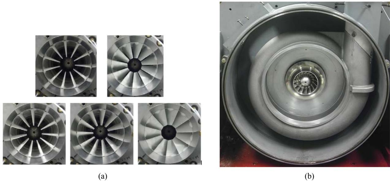
Figure 16. (a) Selective Laser Sintered Inlet Guide Vane Assemblies and (b) 3D Printed Sand Cast Volute Installed in SSTR
