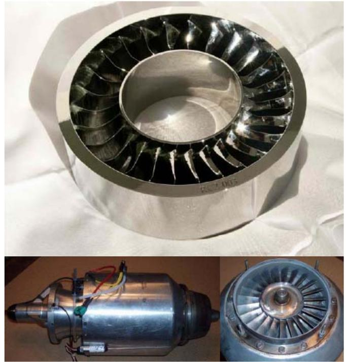
**Figure 2. Flow Straightener for Helicopter Gas Turbine Engine (Above) and Gas Turbine Wheel (Below) (Killian 2013)**
