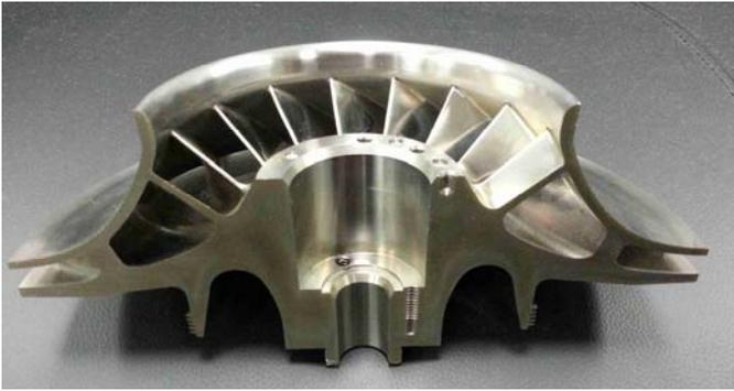
Figure 11. Section View of 2<sup>nd</sup> Generation DMLS Shrouded Impeller Indicating Good Solidity
