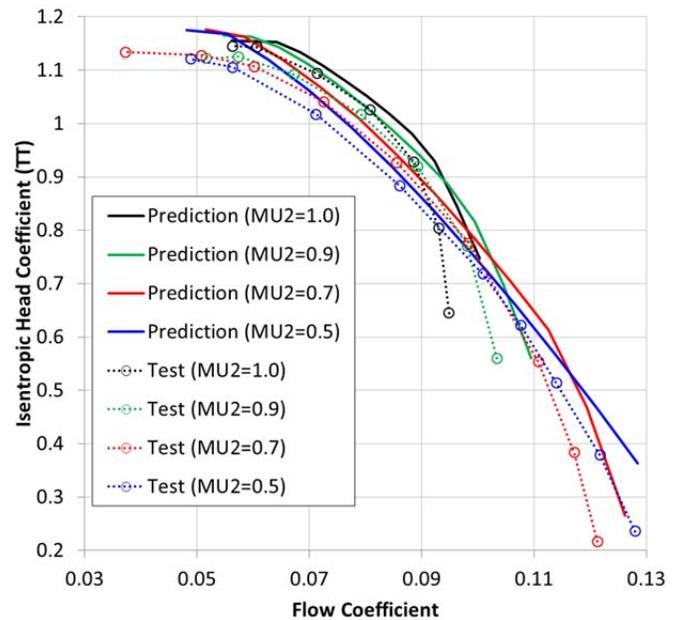
Figure 17. Comparison of Predicted and Tested Head vs. Flow Coefficient
