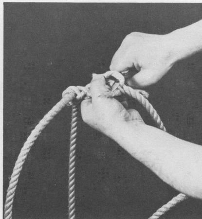
**11.** After each strand has been tucked once, each alternately should be passed over the next strand to it and then tucked under the next one. Continue this procedure until you have tucked each strand several times. Next, dampen the nose piece splice, roll it under your foot on a rough floor, and cut off the loose ends of the strands.
