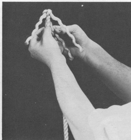
**17.** Draw each strand downward to lay in the same direction as the long rope. Now tuck each strand alternately into the rope as shown in figure 12 until each strand has been tucked several times. Dampen, roll, and then cut off any loose ends to complete the crown.
