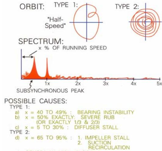
**Figure 9. Subsynchronous Vibration**
