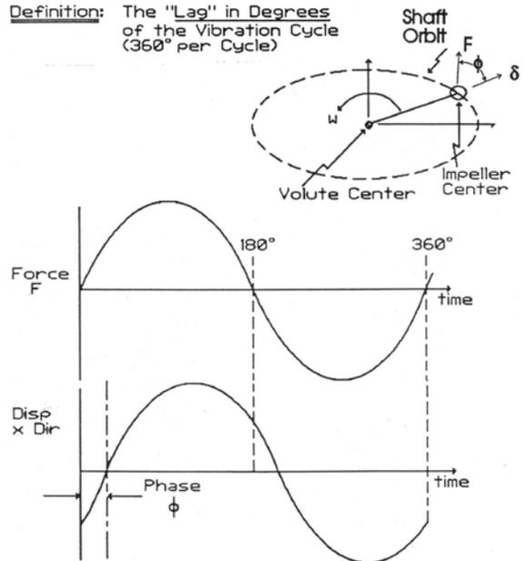
**Figure 2. Definition of Phase Angle**
