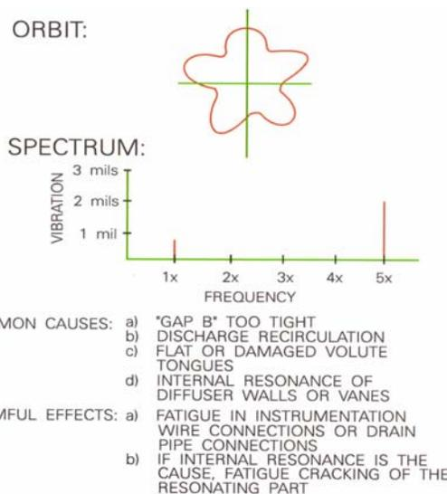
**Figure 12. Vane Pass Vibration**
