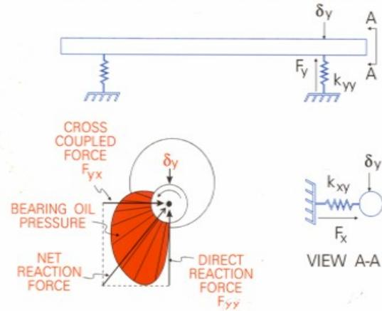
**Figure 10. Cross-Coupled Stiffness Subsynchronous Whirl & Whip**
