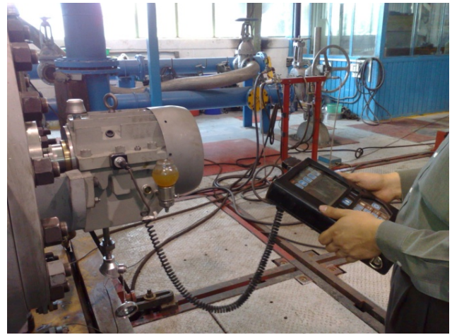
Figure 3. Bearing Housing Vibration Measurement
