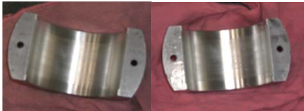
Figure 5. Post-Test Inspection of Hydrodynamic Bearings
