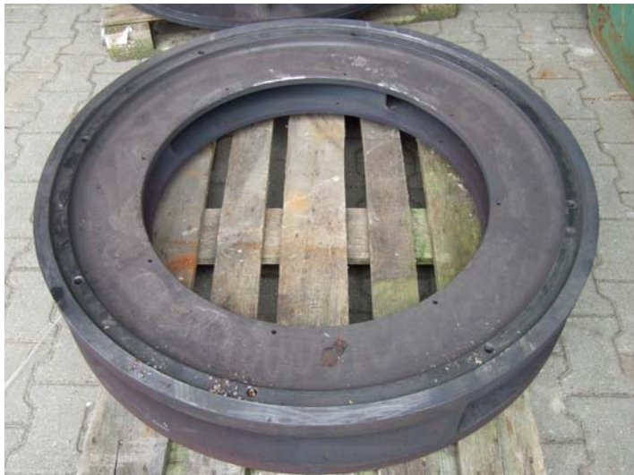
Existing diffuser (4 vanes)
