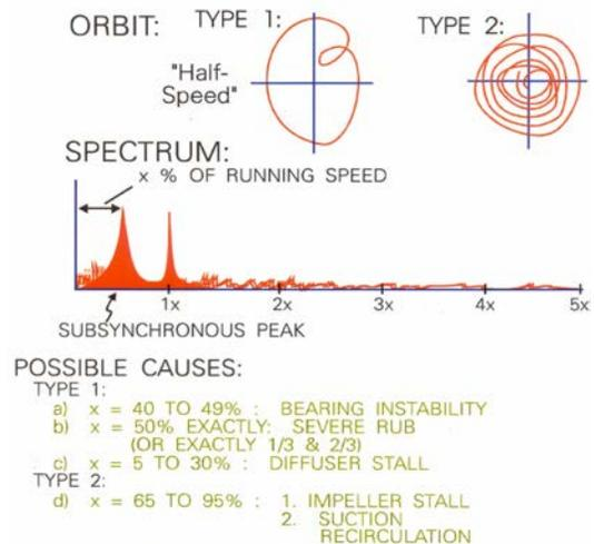
**Figure 9. Subsynchronous Vibration**
