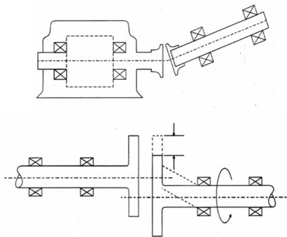
**Figure 6. Illustration of Angular and Offset Misalignment**
