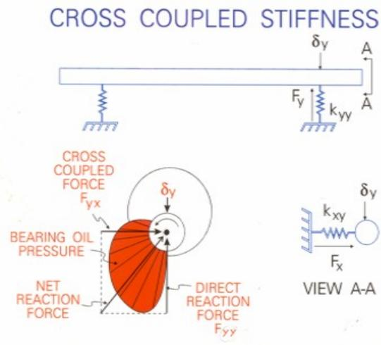
**Figure 10. Cross-Coupled Stiffness Subsynchronous Whirl & Whip**
