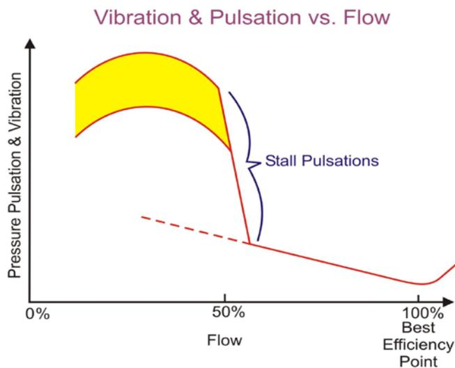
**Figure 11. Effect on Vibration on Off-BEP Operation**
