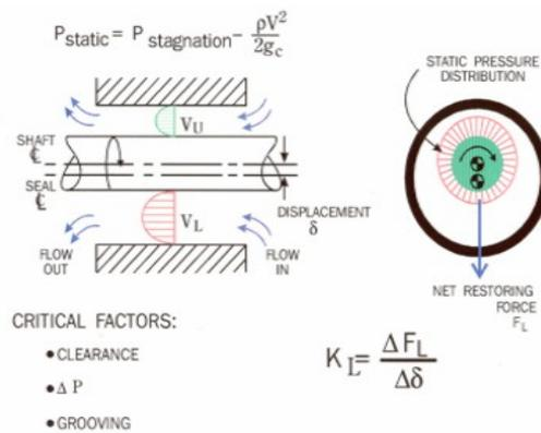
**Figure 14. Illustration of the Lomakin Effect Stiffness  $K_L$  in an Annular Sealing Passage**
