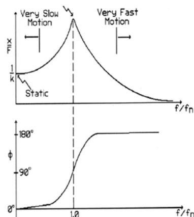
**Figure 3. Relationship of Phase Angle to Frequency
