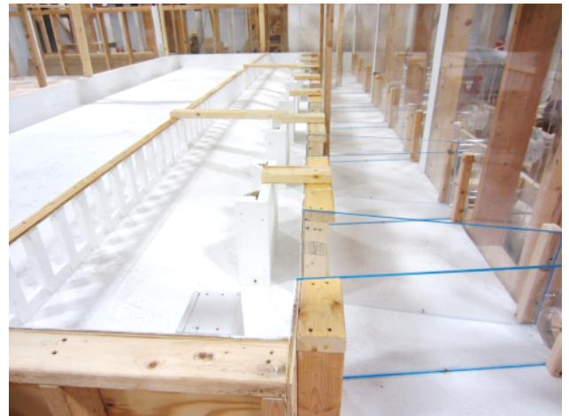
Figure 8. Pump Bays of Physical Hydraulic Model
