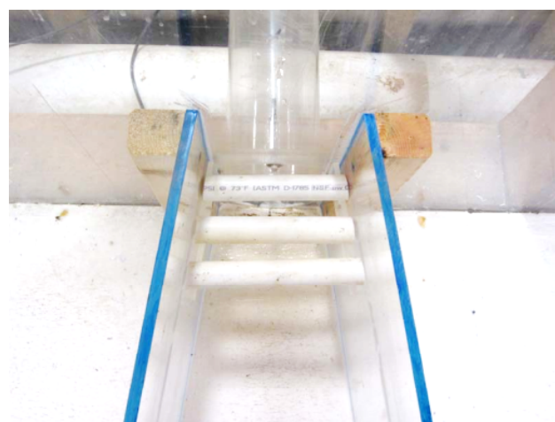
Figure 13. Vortex Suppression Pipes Modification Installed on Model
