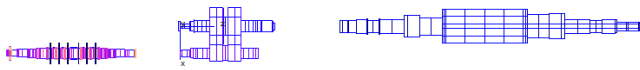
Figure 4 – Outline of the torsional dynamic system. From left to right: compressor, pinion gear (lower center), wheel gear (upper center), electric motor (right).
