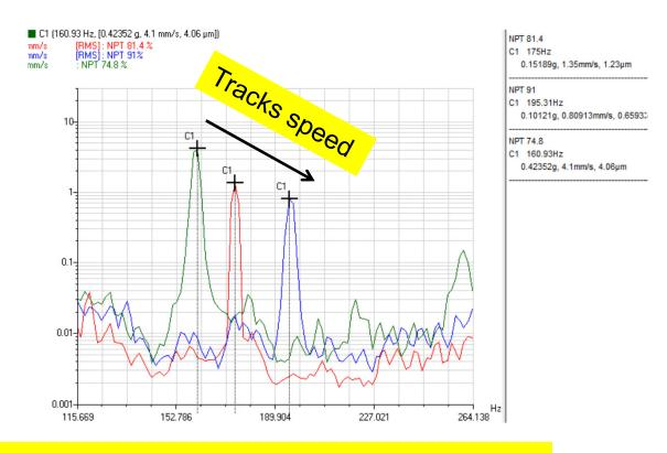
Mechanical and acoustical resonance is ruled out
