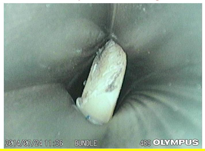
Disassembly of the compressor revealed about 50% of one impeller passage was blocked
