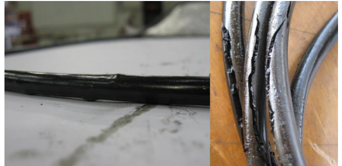
Figure 23 – The process of ED damage begins with visible bubbling of the O-ring (left) that eventually tears (right). Suggest making this two separate figures.
