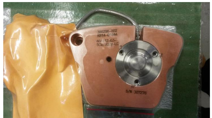
Figure 10. Picture of a thrust bearing pad with load cell.
