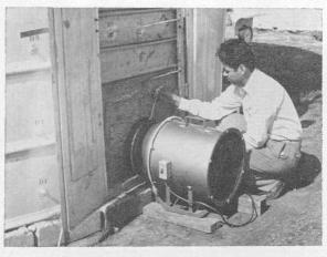
Place a good quality thermometer in a slot in the duct near the bin wall for checking the grain temperature after the fan is started.
