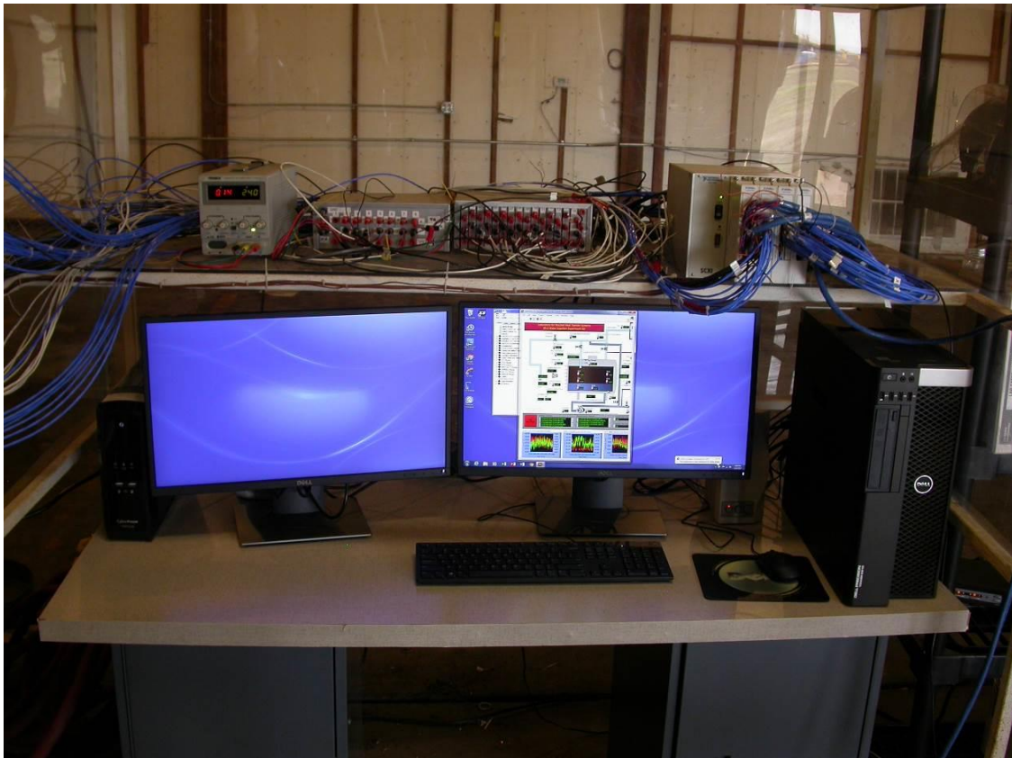
Figure 19: Data acquisition control station.
