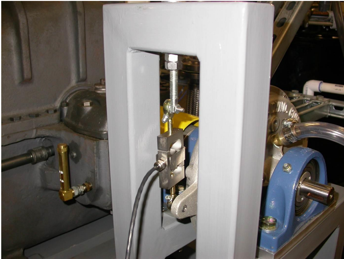
Figure 29: Load cell attachment to dynamometer.
