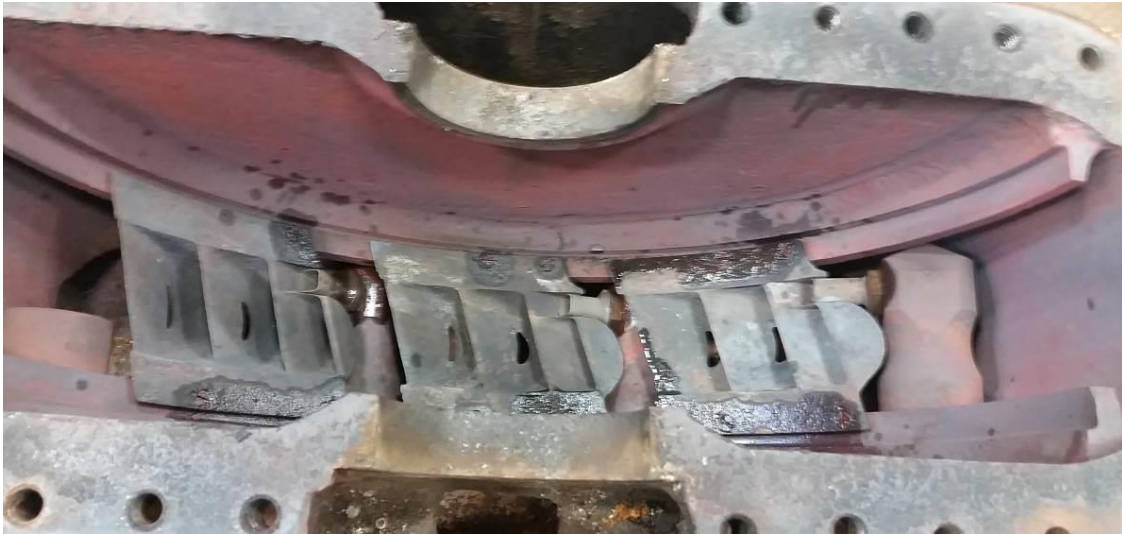
Figure 8: Lower casing, with original nozzles and reversing chambers.
