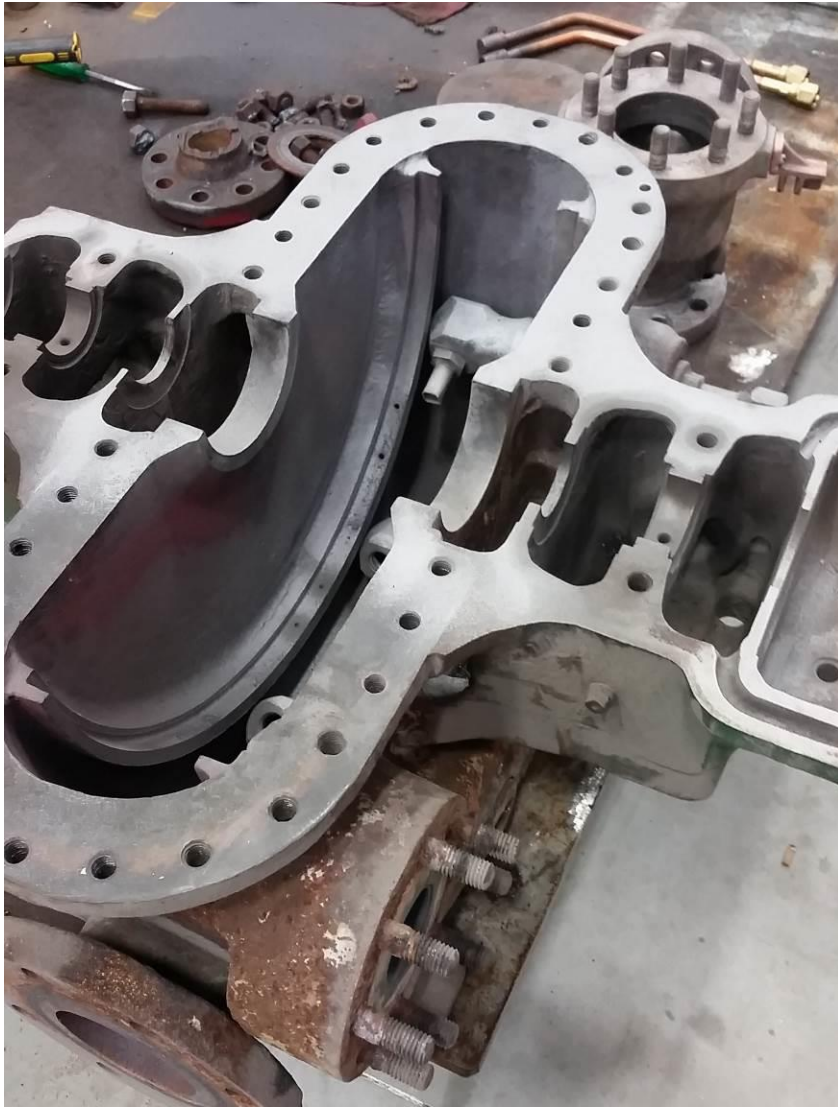
Figure 9: Lower casing, after sandblasting, with two nozzles removed.
