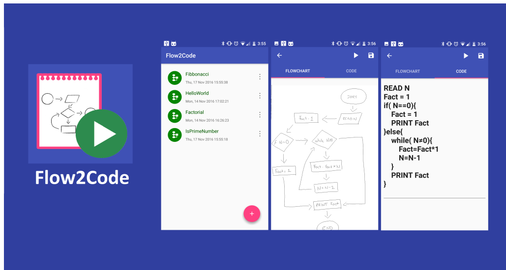
Figure 4.19: This image present the main modules of the mobile application. The first one from left to right enable the management of projects, followed by the recognized flowchart and then the code that was generated from it. The step of taking a picture with the flowchart was not included since the camera itself is outside the scope of the application.
