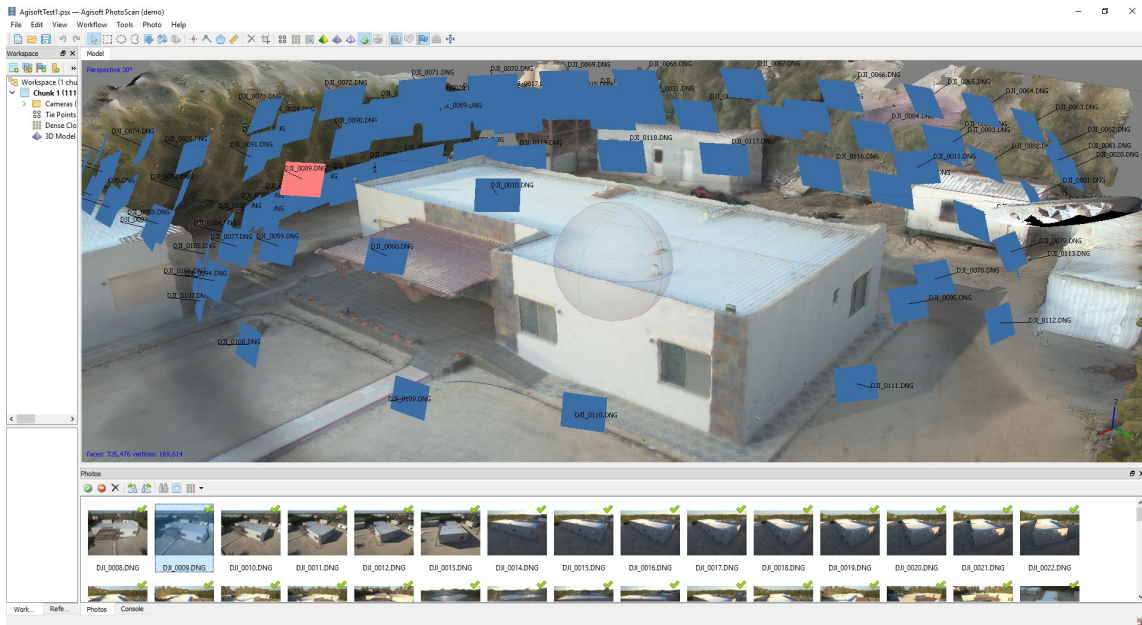
Figure 5. The reconstructed 3D mesh in Photoscan.
