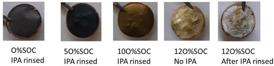
Figure 45. Images of four electrodes at four different SOC for SEM imaging
