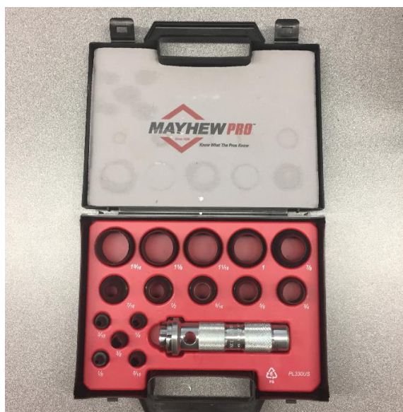
Figure 18. Punch set utilized for creating the electrodes used in coin cells.
