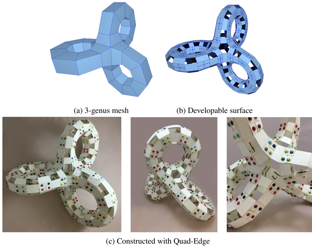
Figure 6.5: 3-genus object constructed with Quad-Edge.
