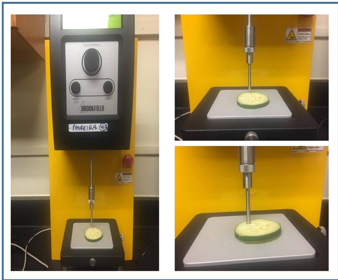
Figure 9. Brookfield CT3 with sample under compression test.
