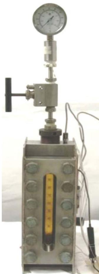
Fig. 2.7. HP/HT see-through cell equipment.
