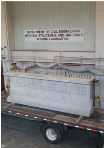
(a) Girder Segments with Lifting Points
