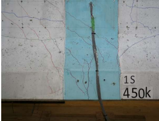
(a) Setup for testing Splice 1
