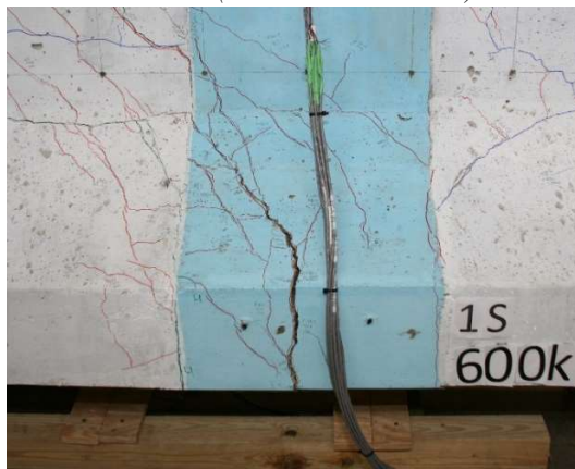
(b) Flexural crack in Splice 1 ( P = 2000 \text{ kN} = 450 \text{ k} )
