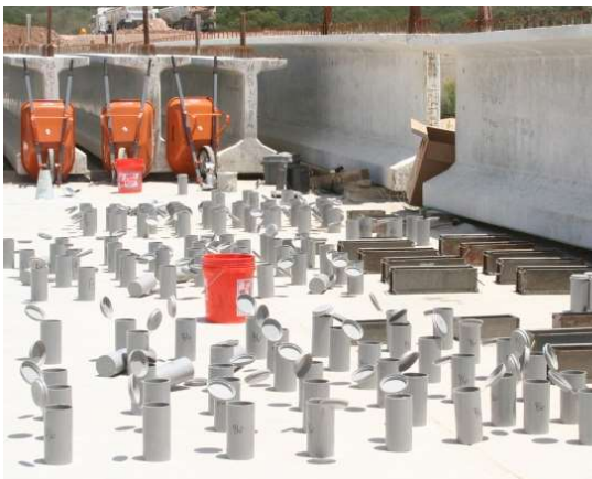
(c) Molds for Hardened Property Samples
