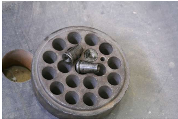
(b) Anchorage Plate and Anchor Wedges
