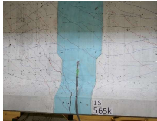
(c) Growth of flexural and shear cracks (d) ( P = 2515 \text{ kN} = 565 \text{ k} )
