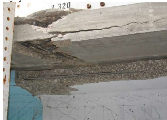
(c) Buckling of deck reinforcement after failure
