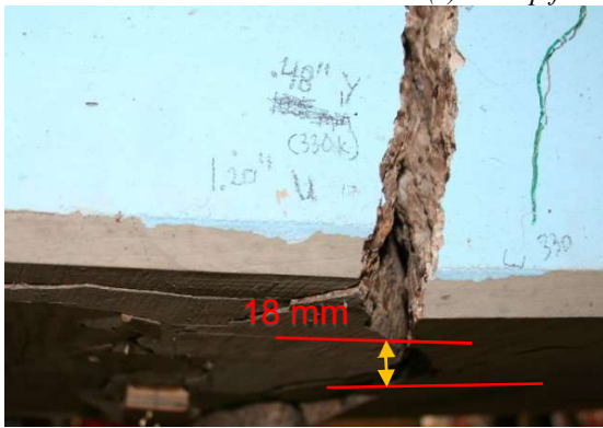
(b) Differential displacement at Splice 2
