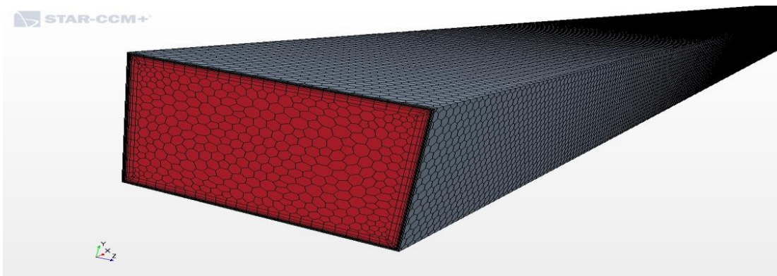
Figure 57. Generated volume mesh for rectangular duct with aspect ratio of 1.5 and hydraulic diameter of d_h = 0.4 m.
