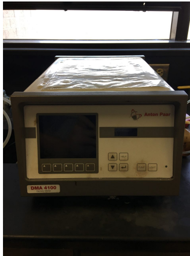
Figure 2.4: A photo of density meter used to study liquid density.
