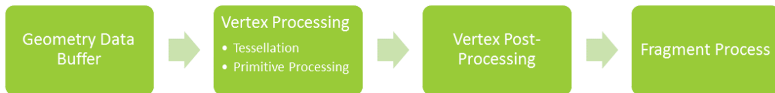
Figure 5.2: Workflow of modern graphics pipeline.
