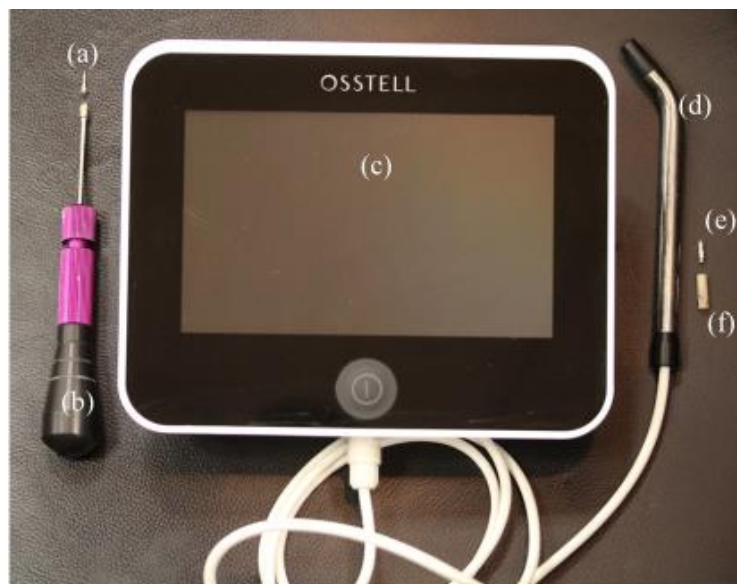
Figure 1. MSI and Osstell IDx Components. (a) Neodent 7mm SLA MSI (b) MSI Hand Driver (c) Osstell IDx (d) Transducer (e) SmartPeg Type A3 (f) SmartPeg Wrench
