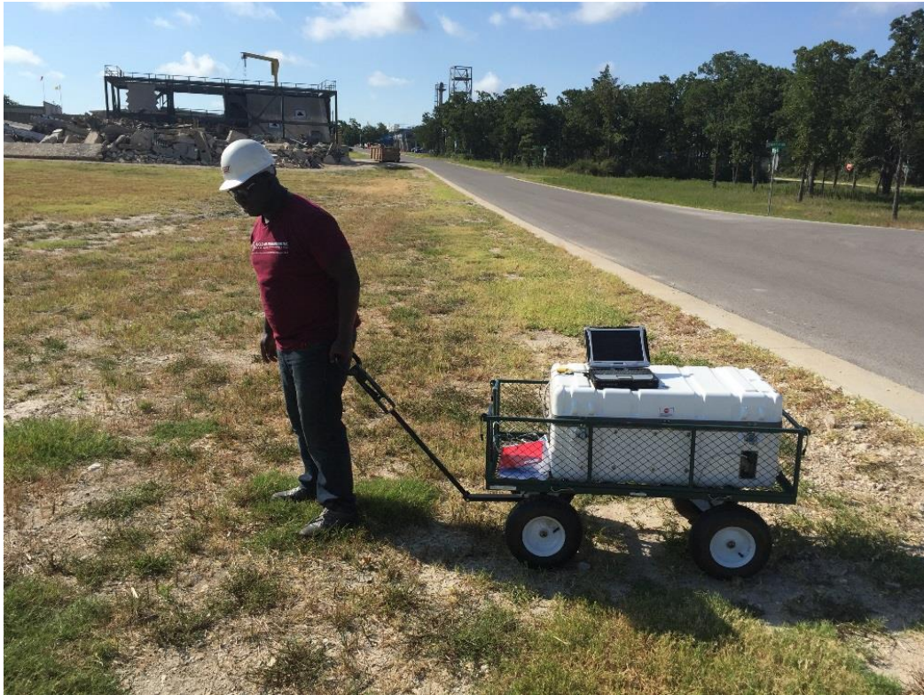
Figure 4. Walkover system configuration used for the DC survey.
