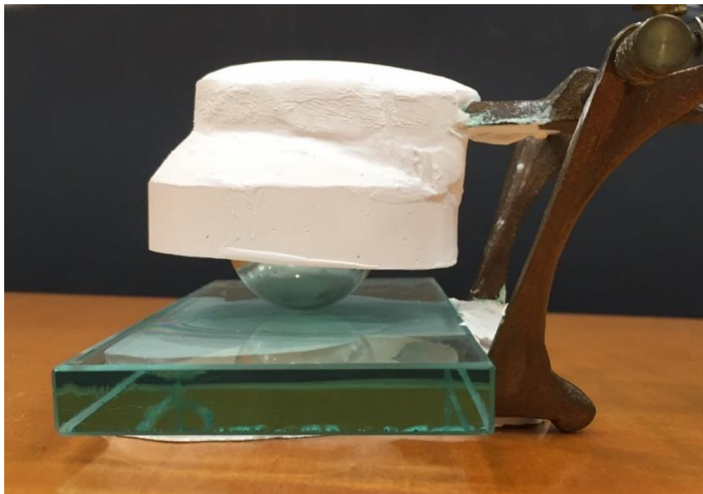
Figure 4: Ball bearing secured to articulator, resting on glass surface
