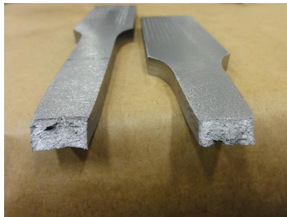
Figure 4-5 – Tensile Test Specimen after testing
