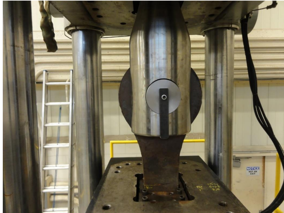
Figure 3-3 – Fatigue Test Setup in 1500 kip frame
