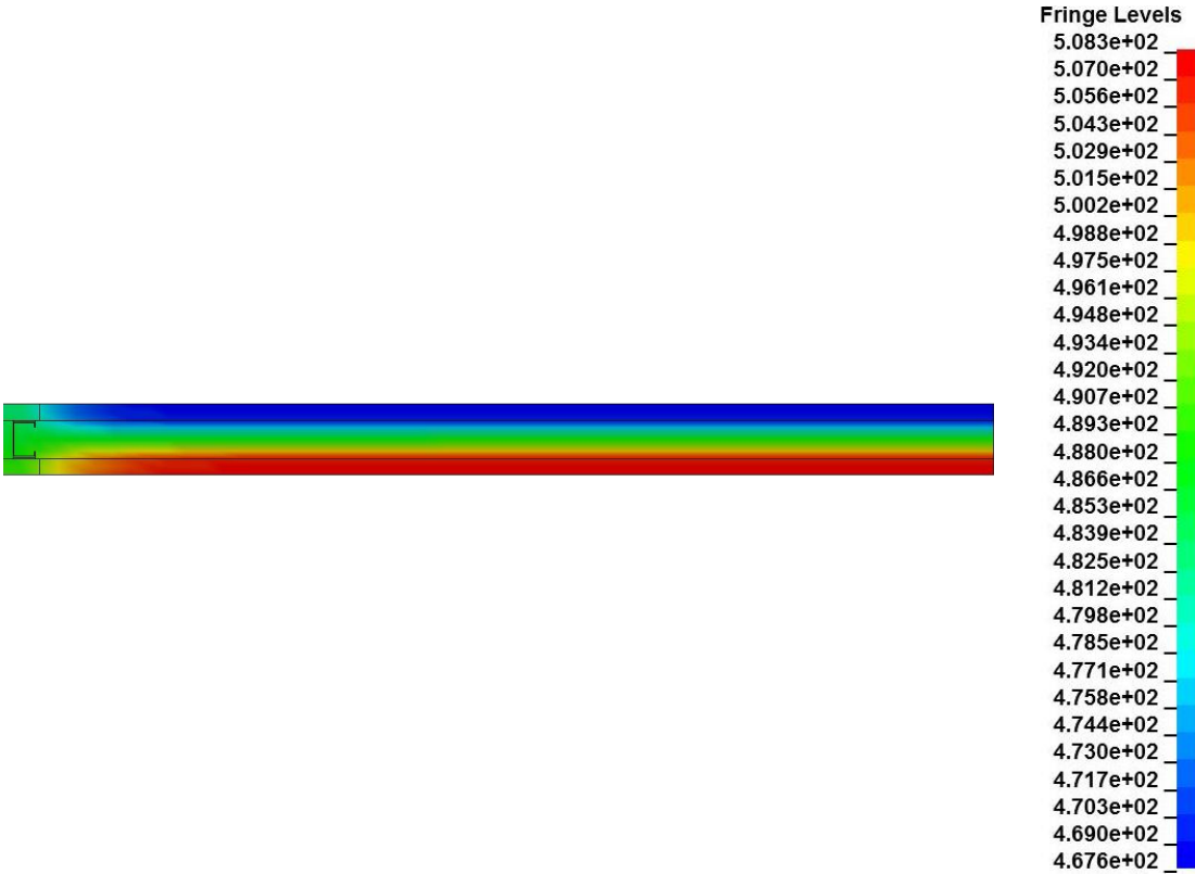
Fig. 35. Steady-State Temperatures for FEA 1
