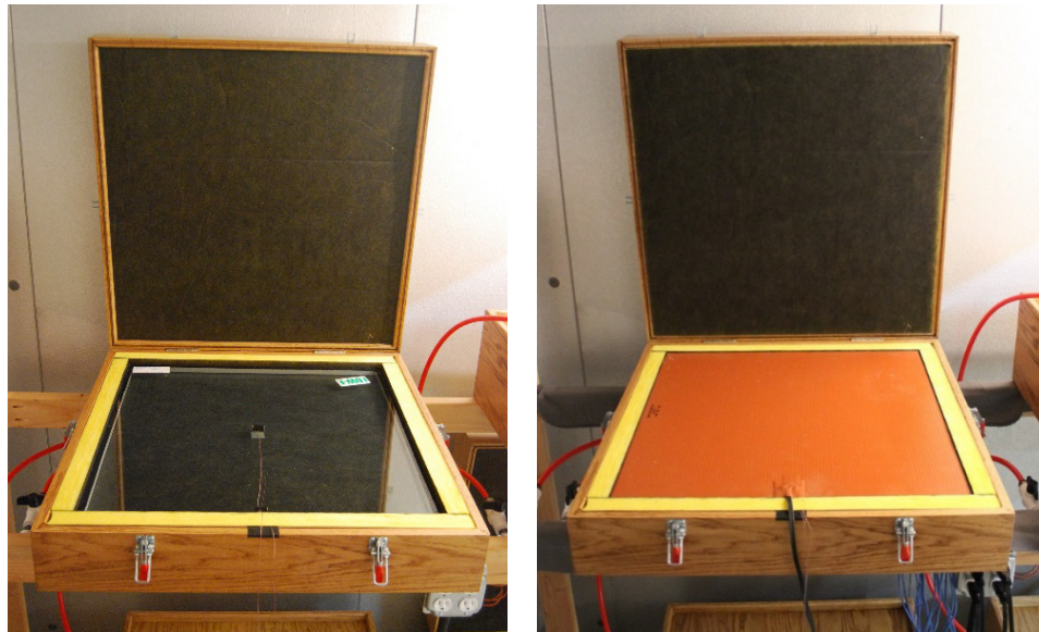
Fig. 87. IG Unit Specimen with Thermocouples Installed
