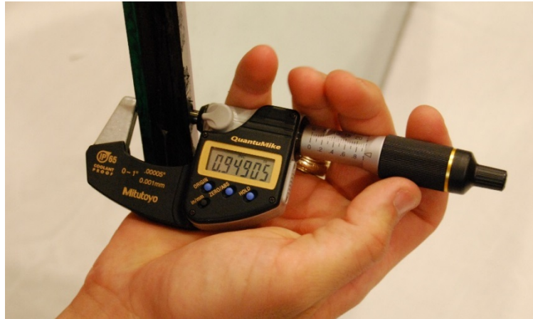
Fig. 82. Measurement of Overall Thickness Using Digital Micrometer
