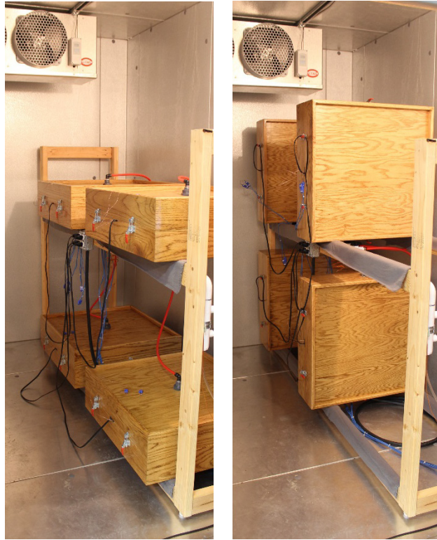
Fig. 91. Specimen Test Rack in the Environmental Test Chamber
