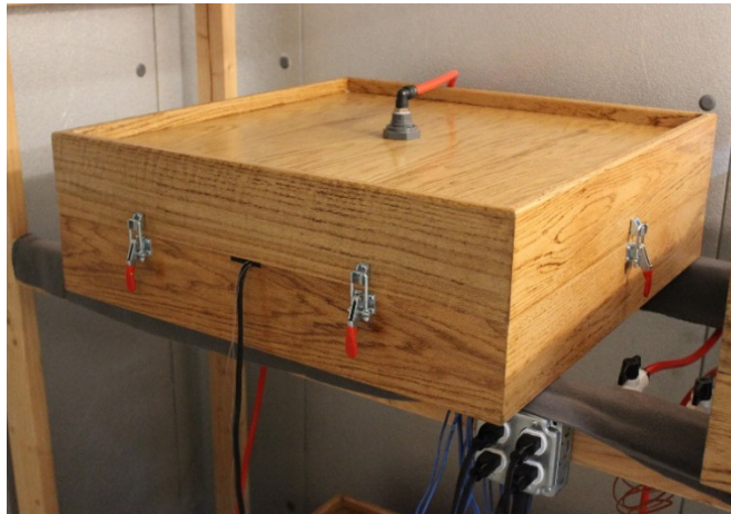
Fig. 86. Insulated Heat Chamber for Determining the CEEC
