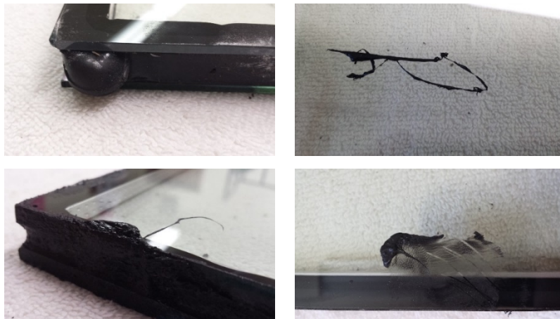
Fig. 80. Extraneous Silicone Shown on Test Specimens
