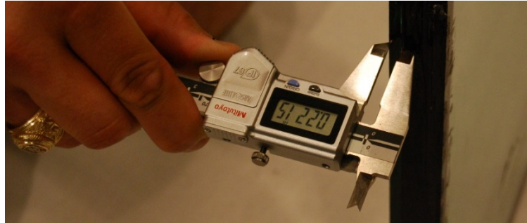
Fig. 83. Measurement of Glass Plate Thickness Using Digital Caliper
