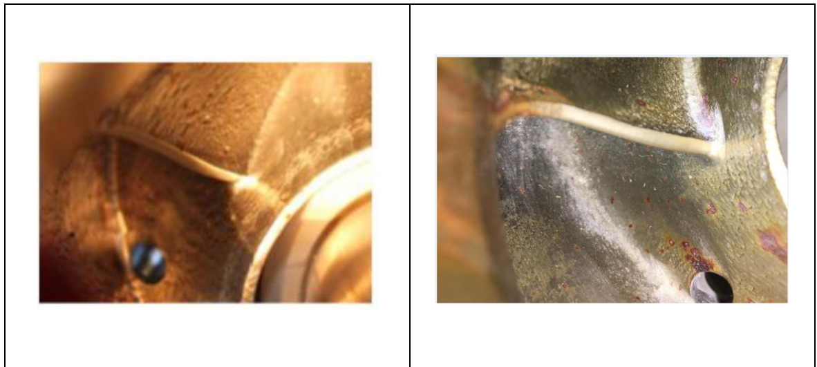
Figure 64 Wear Mark on Leading Edges of Impeller
