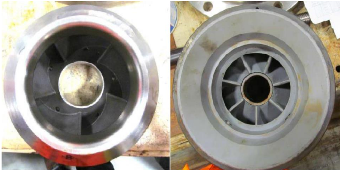
Figure 36 Impeller Suction and Diffuser Discharge Sections, respectively [27]
