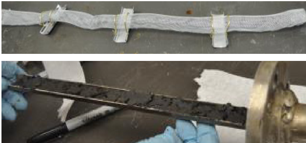
Figure 19: Aluminum mesh and tray soil supports
