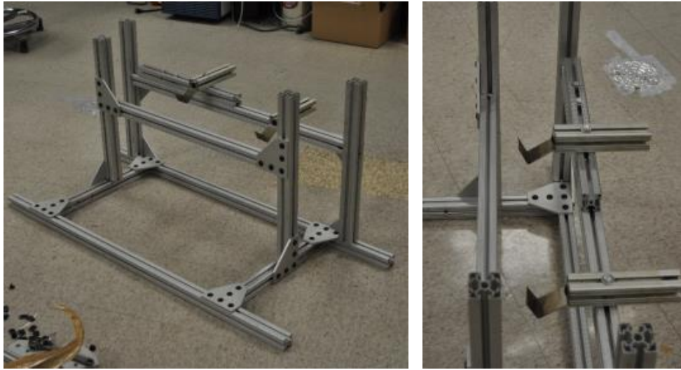
Figure 23: Modified aluminum frame for high-temperature electron beam experiments
