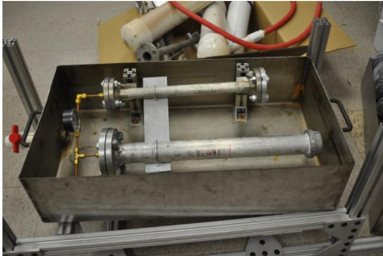
Figure 22: Electron beam reactor in the aluminum tub
